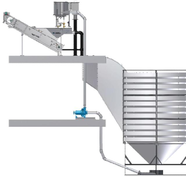
**Figure 6.2: Typical Grit Removal System (Figure Courtesy of Eutek)**
