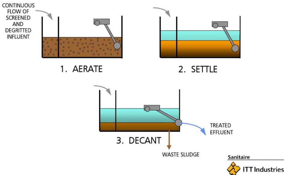
Figure 6.11: SBR System Schematic
