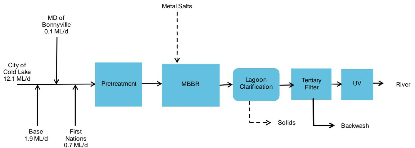
**Figure 6.16: MBBR Process Flow Diagram**
