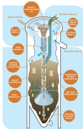
**Figure 6.3: Dynasand Filtration Unit (Figure Courtesy of Parkson)**
