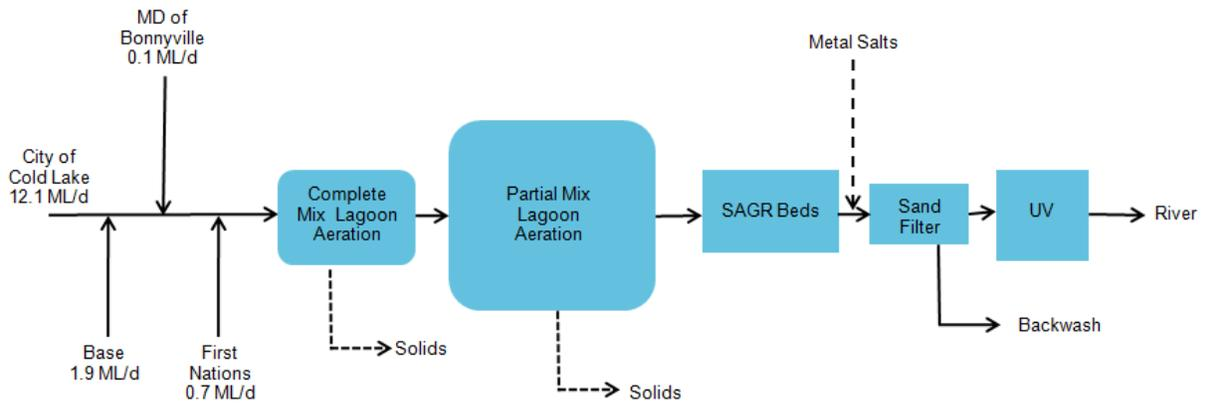
Figure 6.19: SAGR System Process Flow Diagram
