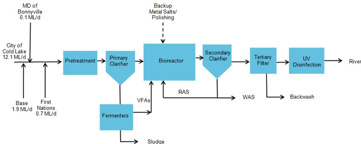
**Figure 6.7: CAS with Chemical Phosphorus Removal Process Flow Diagram**
