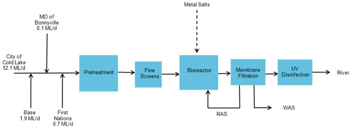
Figure 6.10: Membrane Bioreactor Process Flow Diagram
