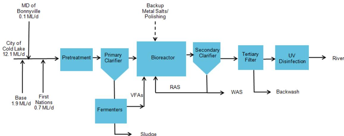
**Figure 6.6: CAS with Biological Phosphorus Removal Process Flow Diagram**
