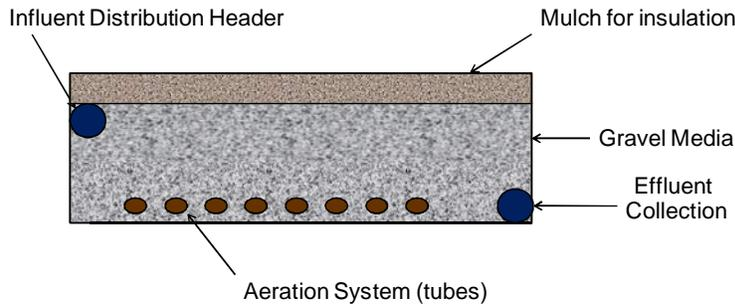
**Figure 6.17: Simplified Schematic of the SAGR System**
