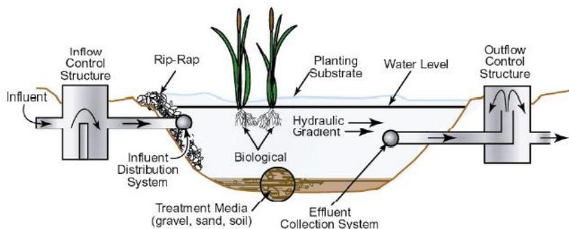
**Figure 6.21: Vegetated Submerged Bed (Horizontal Flow) Schematic**
