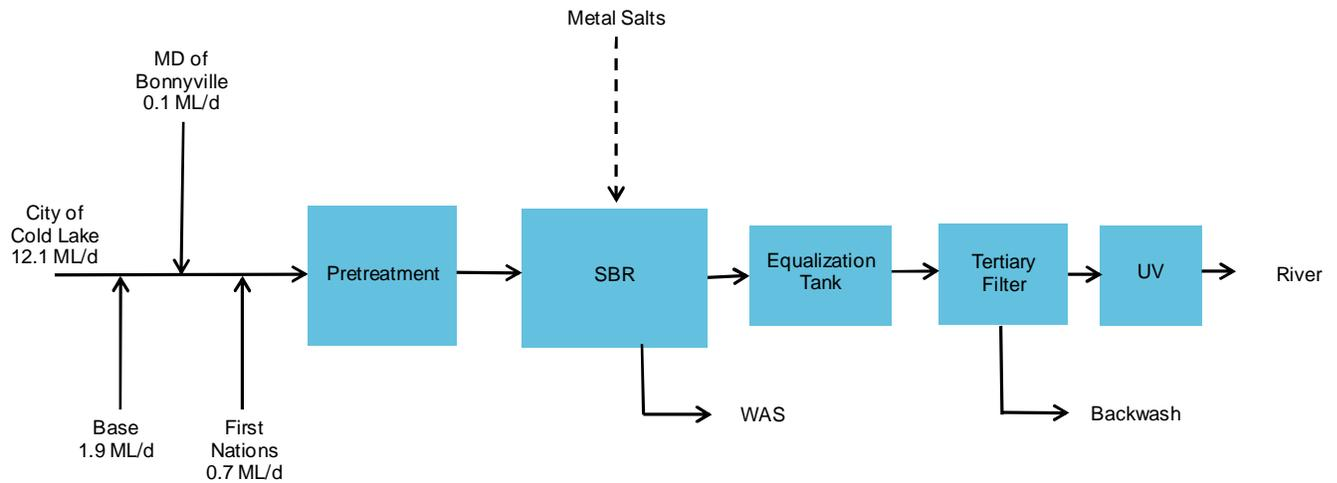
Figure 6.13: SBR Process Flow Diagram
