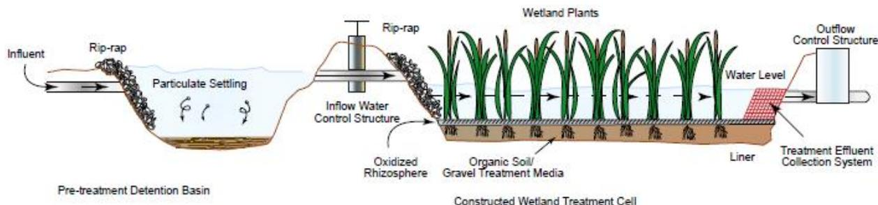
**Figure 6.20: Free Water Surface Wetland Schematic**
