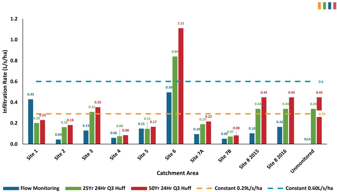
Figure 7.5: Comparison of Infiltration Rates for Each Catchment Area
